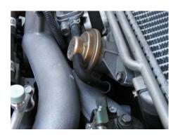
2. Cut through the BOV hose approximately 1" after the bend with a hose cutter or sharp utility knife.
