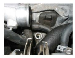
3. Install the block adapter and washer with the 15/16" socket and extension. Torque to approximately 30 lbs. ft.
