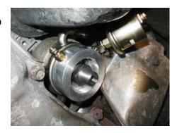
3. Install a new filter and tighten to manufacturer's specifications.
