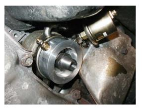
4. Install a new filter and tighten to manufacturer's specifications.
