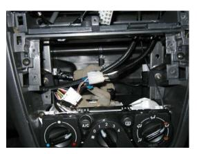
20. Run the illumination harness parallel to the main harness to the right of the center vents. At this point the ends of the main harness, illumination harness, and boost line (if applicable) will be accessible where the clock was installed.
