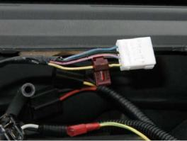
25. Reinstall the stereo, making sure to connect the modular plug, antenna, and ground. Attach the ground wire from the gauge harness as shown.
