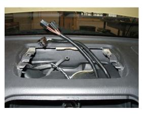
21. Locate the plug that went to the clock. Peel back 1-2" of tape from the wires going into the plug.
