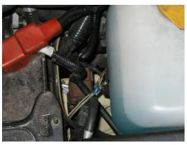
10. Run the wiring harness along the top of the cross member lip and secure with the metal clips. Push the connector(s) onto the spade terminal(s) on the sender(s). Orange is for oil temperature (small sender) and brown is for oil pressure (large sender)
