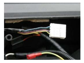
22. Install the red T-Tap on the yellow wire with the green stripe. Position the wire in the slot, fold the T-Tap together, and lock using pliers.
