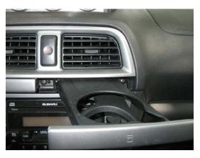
2. Remove the stereo surround trim by pulling it off, starting where the cup holder was removed and working your way around. There are 4 clips that hold it in place. Set trim aside.
